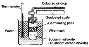
By measuring the movement of the oil drop in the apparatus, what can be investigated?
